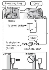
\*DSL/ADSL filter (not supplied) is required if you have DSL/ADSL service.
